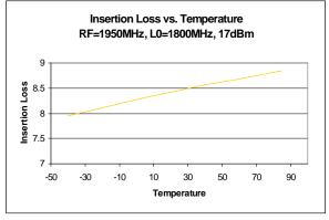
The contour graphs show mixer input TOI and conversion loss over a variety of RF and LO frequencies. These contour graphs can be used to assess the suitability of these mixers over a variety of frequencies of operation. Note that constant IF frequency curves can be overlaid as diagonal lines. Also shown are graphs of TOI and insertion loss vs. temperature. These curves were measured down-converter mode.
