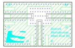
Recommended connectors: Johnson 142-0701-851 SMA end-launch connectors (or equivalent)
